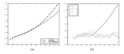
FIG. 5.6. Orthonormality of the Arnoldi vectors for Example 5.3: (a)  $||I_k - V_k^* V_k||^2$  as a function of k for Algorithm 4.4 (symbol  $\triangleleft$ ) and standard GMRES (symbol  $\circ$ ). (b) From bottom to top,  $||I_{m+1} - V_{m-k:k}^* V_{m-k:k}||^2$  as a function of k for m = 1, 2, ..., 5 for Algorithm 4.4.
