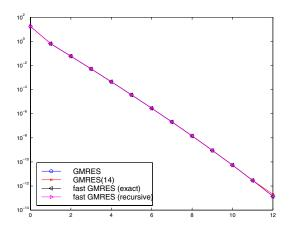
FIG. 5.3. Residual norms for Algorithm 4.4 applied to the data of Example 5.2. For comparison, we show both the norm of the exact residuals  $||b - Ax_k||$  (symbol  $\triangleleft$ ) and the recursive residual norms  $|\gamma_k|$  (symbol  $\triangleright$ ), which are of the same size. The norm of the residuals  $r'_k$  obtained by standard GMRES (symbol  $\circ$ ) and by restarted GMRES(14) (symbol  $\times$ ) are also displayed.
