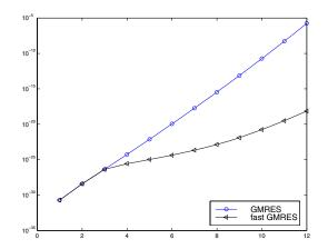
FIG. 5.4. Orthonormality of the Arnoldi vectors for Example 5.2:  $||I_k - V_k^* V_k||^2$  as a function of k for Algorithm 4.4 (symbol  $\triangleleft$ ) and standard GMRES (symbol  $\circ$ ).
