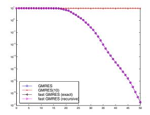
FIG. 5.1. Residual norms for Algorithm 4.4 applied to the data of Example 5.1. For comparison, we show both the norm of the exact residuals  $||b - Ax_k||$  (symbol  $\triangleleft$ ) and the recursively computed residual norms  $|\gamma_k|$  (symbol  $\triangleright$ ), as well as the norm of the residuals  $r'_k$  (symbol  $\circ$ ) obtained by standard GMRES, which are all of the same size. In contrast, restarted GMRES(10) (symbol  $\times$ ) fails to converge.
