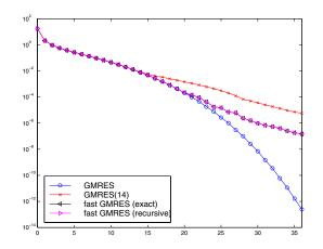
FIG. 5.7. Residual norms for Algorithm 4.4 applied to the data of Example 5.3. For comparison, we show both the norm of the exact residuals  $||b - Ax_k||$  (symbol  $\triangleleft$ ) and the recursive residual norms  $|\gamma_k|$  (symbol  $\triangleright$ ), which are of the same size, and smaller than those obtained by restarted GMRES(14) (symbol  $\times$ ). The norms of the residuals  $r'_k$  obtained by the standard GMRES (symbol  $\circ$ ) are much smaller for  $k \geq 30$ .
