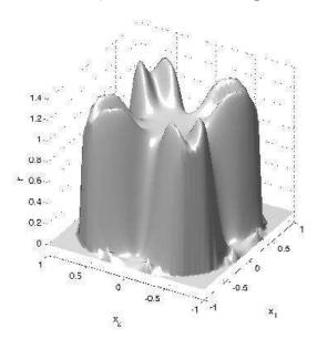
${\it Fig.~4.12.}$  Positive polynomial approximation of degree 20 of the indicator function of the folium surface.
