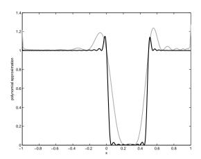
Fig. 4.7. Positive polynomial approximation of degree 100 of the indicator function  $1-I_{[0,\frac{1}{2}]}$  in the Chebyshev basis (black) and power basis (gray).
