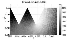
FIG. 7.4. Temperature at t = 0.58 s for the free optimization.
