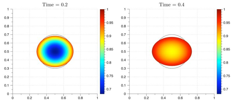
**Fig. 4.6.** Time values from the computed solution of nonlinear advection-reaction-diffusion equations solved on a moving boundary. The initial boundary is a circle indicated by a solid black line. The grid size is  $200 \times 200$ .
