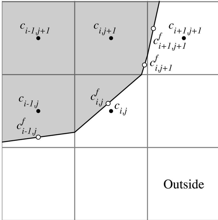
**Fig. 3.1.** The solid line indicates a piecewise linear approximation to the zero level set of the signed distance function. The black points labeled  $c_{i,j}$  indicate values that lie on a Cartesian grid. White points labeled  $c_{i,j}^f$  indicate values associated with the boundary.
