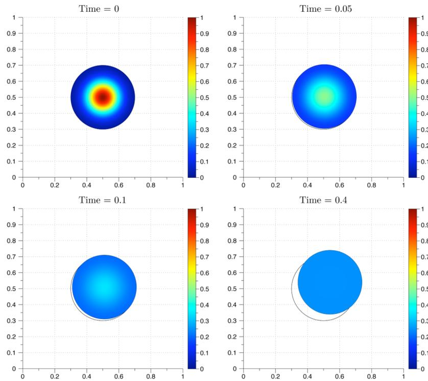
**Fig. 4.1.** Time values from the computed solution of an advection-diffusion equation solved on a circle with Gaussian initial conditions. The diffusion coefficient for this simulation was 0.05. The grid size is  $200 \times 200$ . The initial boundary is the circle indicated by a solid black line.
