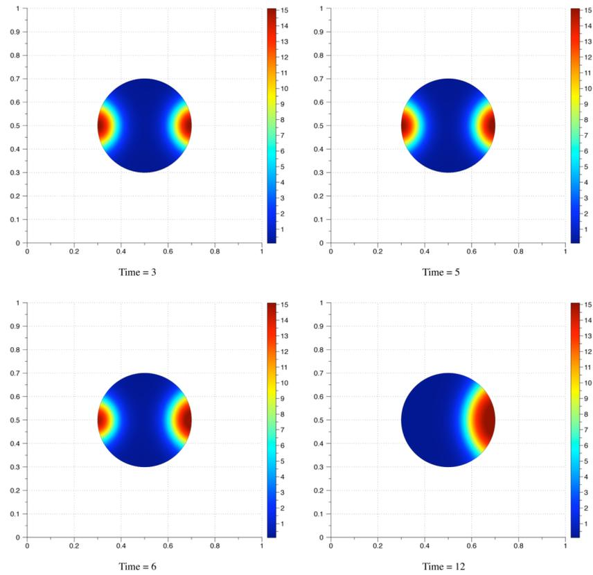
**Fig. 5.3.** Time values for  $[R_2]$  in the substrate depletion model with two initial perturbations and  $U \vec{=}$  0. The grid size used was  $150 \times 150$ .
