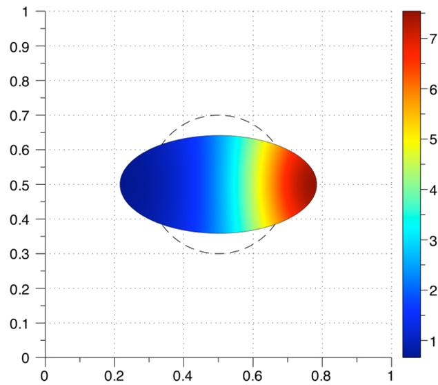
**Fig. 5.1.** Concentration of  $R$  at  $t=35$ . The initial geometry is indicated by a dashed line. The grid size used was  $100 \times 100$ .
