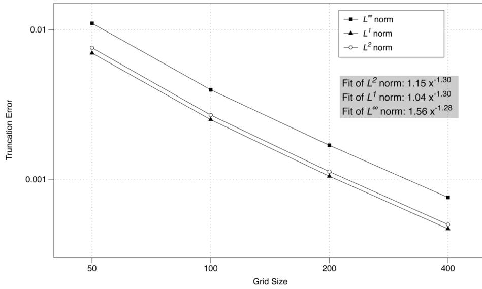
**Fig. 4.4.** Truncation error for nonlinear advection-reaction-diffusion equations at the time value of 0.4.
