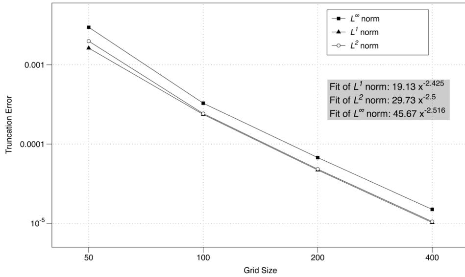
**Fig. 4.2.** Truncation error for the diffusion equation at the time value of 0.4.
