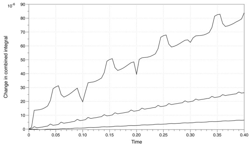
**Fig. 4.5.** Numerical integral of  $C'_i(x, y, t) + C'_d(x, y, t)$  subtracted from the initial value. The top plot is for a grid size of  $100 \times 100$  followed by  $200 \times 200$  and  $400 \times 400$  on the bottom.
