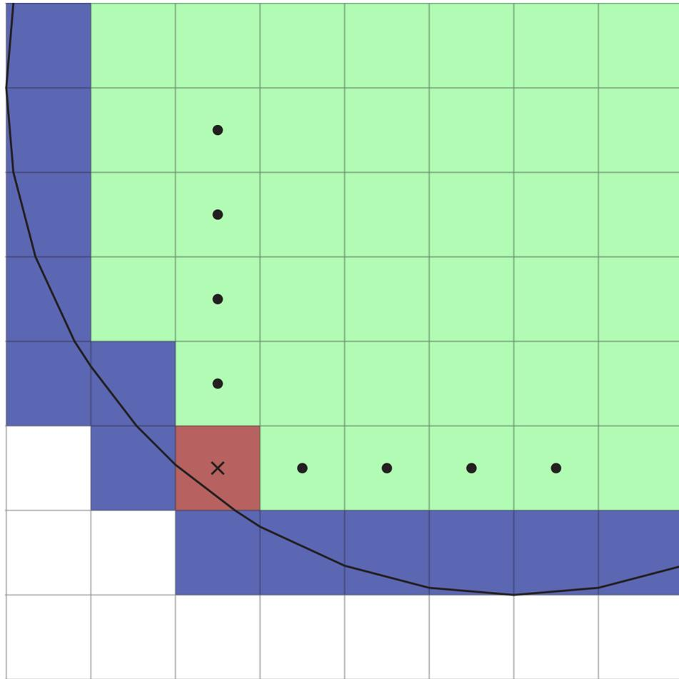
**Fig. 3.4.** Interpolation diagram. Interior values are colored green. Cut cell values are colored blue. Circles mark the interior points used to interpolate at the point marked with a cross.
