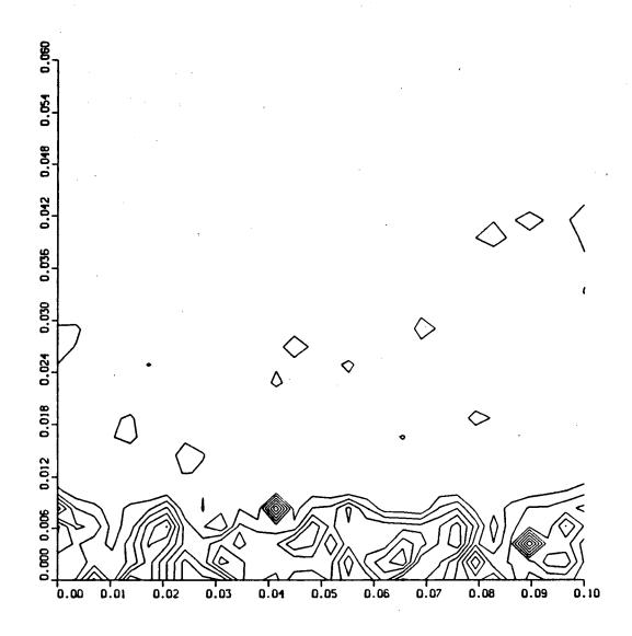
Figure 12. Contours of the y component of vorticity in the y, z plane for x = 1.4.
