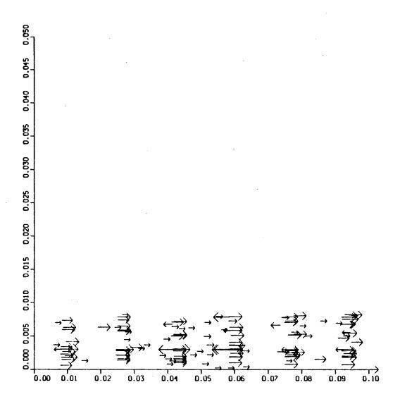
Figure 5. Vorticity in the y, z plane for x = 1.
