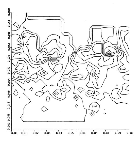
Figure 9. Contours of the z component of vorticity in the y, z plane for x = 1.4.
