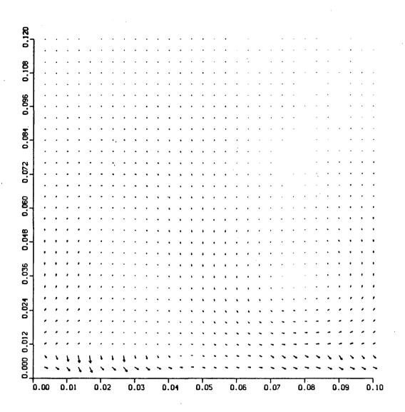
Figure 3. Velocity field in the y, z plane for x = 1.4.
