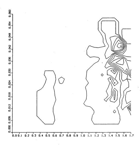
Figure 7. Contours of the z component of vorticity in the x, z plane for y = q/2.
