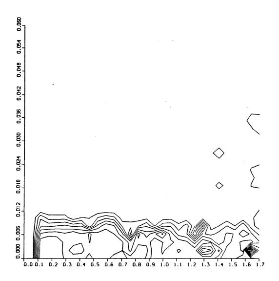
Figure 10. Contours of the y component of vorticity in the x, z plane for y = q/2.
