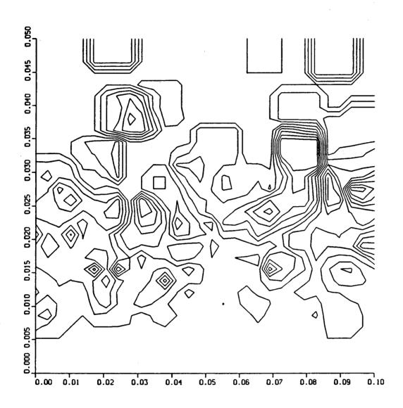
Figure 8. Contours of the z component of vorticity in the y, z plane for x = 1.
