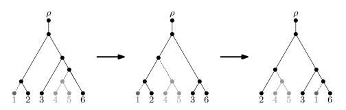
Figure 2: Two rSPR operations, each of which moves one grey subtree. The leftmost and rightmost trees are rSPR distance two apart.
