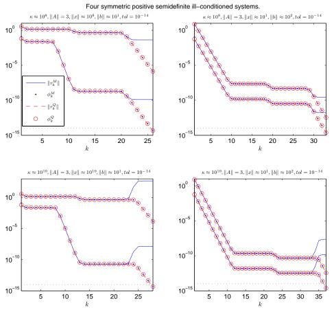
FIG. 8.2. Solving Ax = b with semidefinite A similar to an example of Sleippen et al. [47].  $A = Q \operatorname{diag}([0_5, \eta, 2\eta, 2; \frac{1}{789}; 3])Q$  of dimension n = 797, nullity 5, and norm ||A|| = 3, where  $Q = I - (2/n)ww^T$  is a Householder matrix generated by  $v = [0_5, 1, \dots, 1]^T$ , w = v/||v||. These plots illustrate and compare the effect of rounding errors in MINRES and MINRES-QLP.
