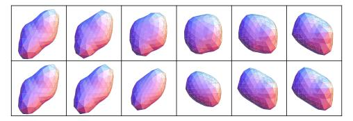
FIGURE 15. Large deformation of a shape for  $\Phi = \text{Vol}$  and  $\Phi = e^{\text{Vol}}$ . 20 timesteps and a triangulation with 500 triangles were used. Time progresses from left to right.
