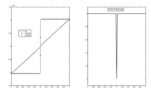
Note that, when we use the CGFEM the discrete solution is close to the function y = x which is a solution of (8.50) with  $p \equiv 2$ , that means that this method needs a smaller step in order to see the points where p is close to one.
