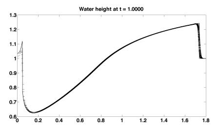
Fig. 3.9. Solution for the 2D radial dam-break problem on a grid with  $500 \times 500$  cells, plotted as a function of radius.
