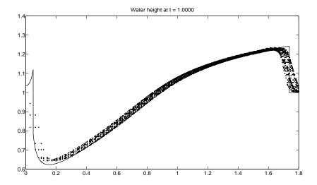
Fig. 3.8. Solution for the 2D radial dam-break problem on a grid with 125 × 125 cells, plotted as a function of radius.
