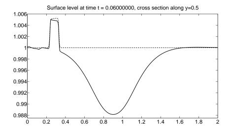
Fig. 3.11. Surface level h + b along a cross section at y = 0.5 and time t = 0.06. Solid line: f-wave Riemann solver and component-wise reconstruction; dashed line: f-wave Riemann solver and f-wave-slope reconstruction.
