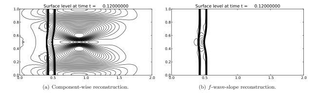
Fig. 3.10. Contour of the surface level h+b at time t=0.12 computed with component-wise reconstruction and f-wave-slope reconstruction. Contour levels: 0.99942:0.000238:1.00656.
