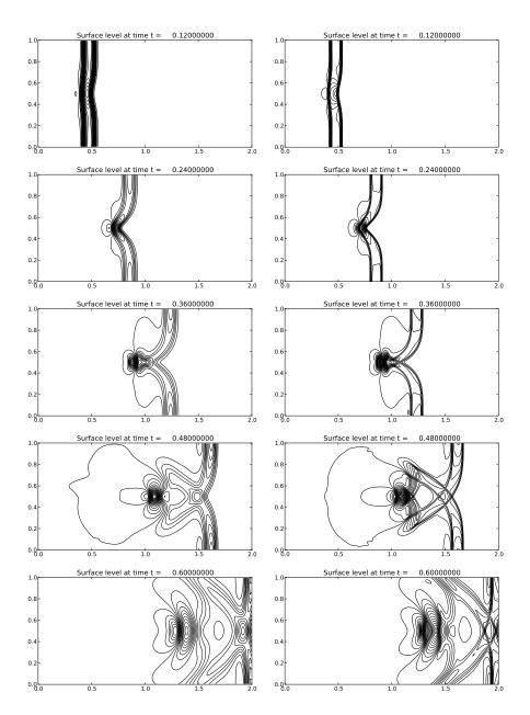
Fig. 3.12. Contour of the surface level h+b. f-wave-slope reconstruction. 30 uniformly spaced contour lines. t=0.12 from 0.99942 to 1.00656; t=0.24 from 0.99318 to 1.01659; t=0.36 from 0.98814 to 1.01161; t=0.48 from 0.99023 to 1.00508; t=0.6 from 0.995144 to 1.00629. Left: results with a  $200\times100$  cells. Right: results with a  $600\times300$  cells.
