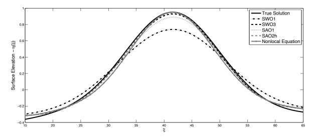
Figure 6: Wave tank comparisons of the reconstructed surface elevation with surface height measurements for  $h = 5.05 \, cm$ . This corresponds to Experiment #1 in Table 8.
