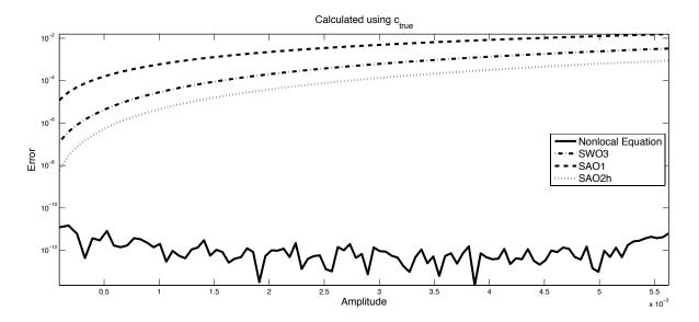
Figure 3: Plot of the relative error (60) in the reconstructed surface elevation  $\eta_r$  as a function of the amplitude of  $\eta_{true}$  using the true value of the wave speed c. The asymptotic approximation SAO2 is not included in this figure. It is more costly to compute than its heuristic counterpart SAO2h, which yields better results.
