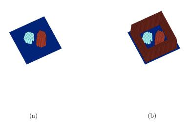
FIGURE 5.1. Visualization of the relative dielectric permittivity  $\varepsilon_r$  of the numerical phantoms utilized for the first set of scattering experiments. The phantoms are piecewise homogeneous and purely dielectric, i.e., non-absorbing.
