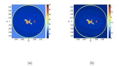
FIGURE 5.3. Numerical phantom of the breast slice utilized in our scattering simulations, performed at a frequency of f = 3 GHz. Panel (a): pixel values of the relative dielectric permittivity  $\varepsilon_r$ . Panel (b): pixel values of the conductivity  $\sigma$ . In both panels, the tumoral mass is the small disk centered at (0.02,0) m and with a diameter of 0.5 cm.
