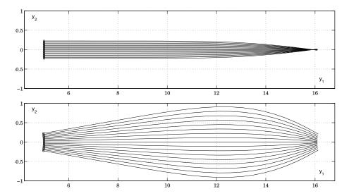
Fig. 2. Illustration of canonical relations  $\chi$  (top) and  $\check{\chi}$  (bottom) of operators F and  $\check{F}$  associated with a half-wave equation: (bi-)characteristics ("rays") in y for initial conditions ( $x_2 = x_{2,0}, \ \xi = \xi_0$ ) and ( $\tilde{x}_2 = \tilde{x}_{2,0}, \ \tilde{\xi} = \tilde{\xi}_0$ ), respectively, for evolution through a low velocity lens (see Section 5). The black circles on the left indicate the conjugate points corresponding to the initial conditions.
