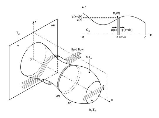
Figure 1: Scheme of the axisymmetric fin
