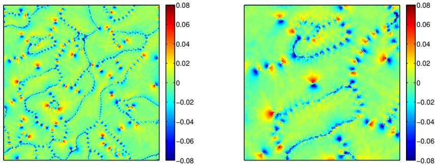
FIGURE 16. Left: The local volume distortion estimate  $\text{Vol}(b)$  of the phase field crystal image example in Figure 15 and its zoomed-in result. The color limits of these two images are set to be 0.08 and  $-0.08$ .
