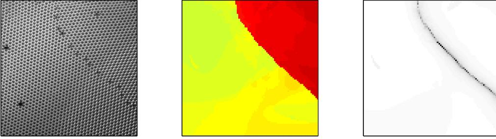
FIGURE 13. Left: A photograph of a bubble raft with strong reflections and point dislocations (courtesy to Don Stone, copyright 2009 Board of Regents of the University of Wisconsin System). Its size is  $476 \times 476$  pixels. Middle and right: The weighted average angle  $\text{Angle}(b)$  and the boundary indicator function provided by Algorithm A. Primary implementation parameters:  $s = t = 0.5$ ,  $d = 0.5$ .
