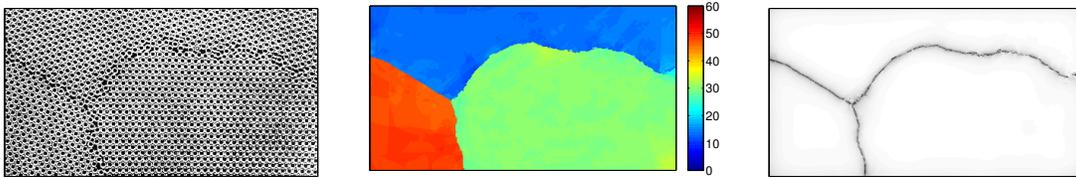
FIGURE 12. Left: A photograph of a bubble raft with large disorders and blurry boundaries. Courtesy to Barrie S. H. Royce in Princeton University. The image size is  $223 \times 415$ . Middle and right: The weighted average angle  $\text{Angle}(b)$  and the boundary indicator function provided by Algorithm A. Primary implementation parameters:  $s = t = 0.5$ ,  $d = 1$ .
