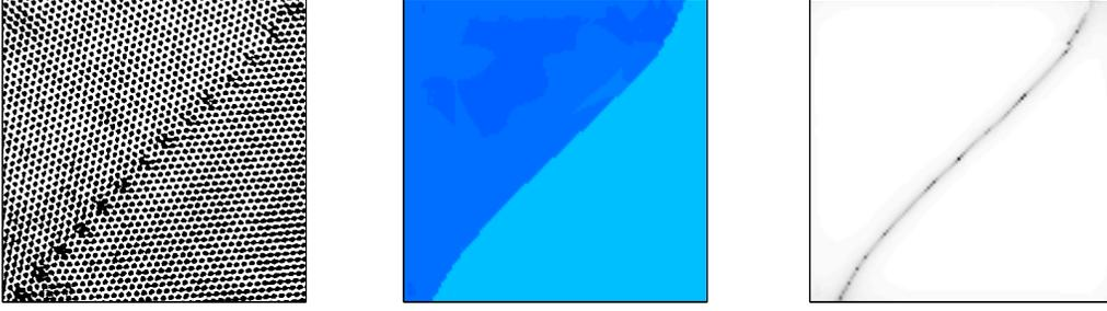
FIGURE 11. Left: A TEM-image of size  $420 \times 444$  pixels in GaN. Courtesy of David M. Tricker (Department of Material Science and Metallurgy, University of Cambridge). Middle: The weighted average angle  $\text{Angle}(b)$  provided by Algorithm A. Right: The boundary indicator function  $\text{BD}(b)$  provided by Algorithm A. Primary implementation parameters:  $s = t = 0.5$ ,  $d = 0.5$ .
