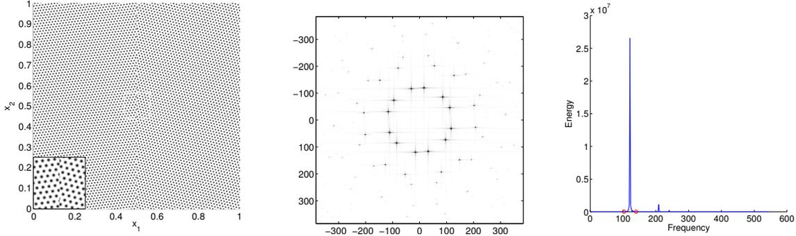
FIGURE 3. Left: An undeformed example of two hexagonal grains with a vertical line boundary. Middle: Its Fourier power spectrum. The number of dominant local wave vectors is 12 due to the superposition of spectrum of the two grains. Right: Its radially average Fourier power spectrum with the identified most dominant energy bump indicated by two red circles.
