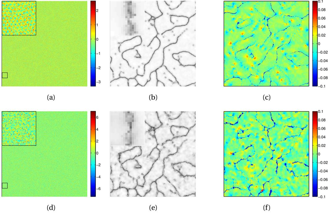
FIGURE 17. Analysis results of noisy phase field crystal images provided by Algorithm *B*. First row: Results of noisy data with Gaussian white noise  $0.5\mathcal{N}(0, 1)$ . Second row: Results of noisy data with Gaussian white noise  $1.4\mathcal{N}(0, 1)$ . First column: input images. Second column: detected grain boundaries and isolated defects. Third column: distortion volume. Zoomed-in images show that our method can still identify isolated defects even if noise is heavy.
