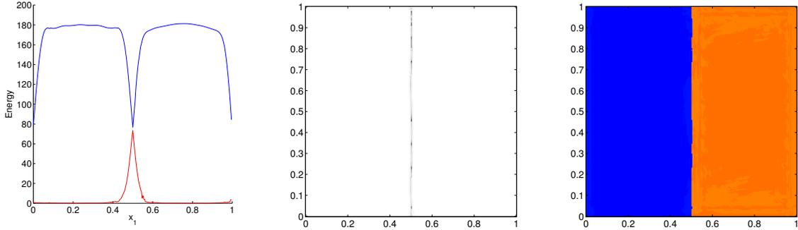
FIGURE 5. Left: The total energy function  $TE_1(b)$  in blue and  $TE_2(b)$  in red for fixed  $b_2 = 0.5$ . Middle: The boundary indicator function  $BD(b)$ . Right: The weighted average angle  $\text{Angle}(b)$  as an approximation of crystal rotations. The real crystal rotations are 15 degrees on the left and 57.5 degrees on the right.
