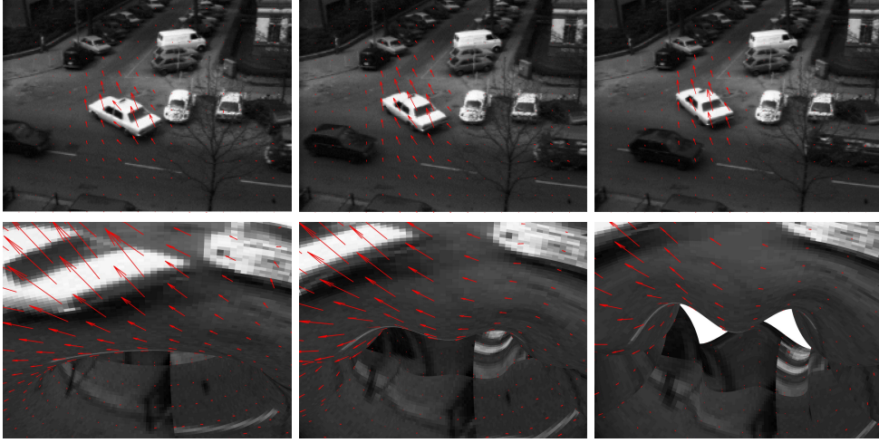
Figure 2: The optical flow vector field resulting from Experiment I at frames 1, 10, and 19. Top row: the pull back of the vector field. Bottom row: the vector field on the moving surface. The vectors have been scaled for better visibility.
