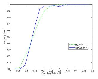
Fig. 4. Recovery rate of piecewise second-order polynomial functions as a function of the sampling rate m/d for the methods BGAPN and SSCoSaMP.
