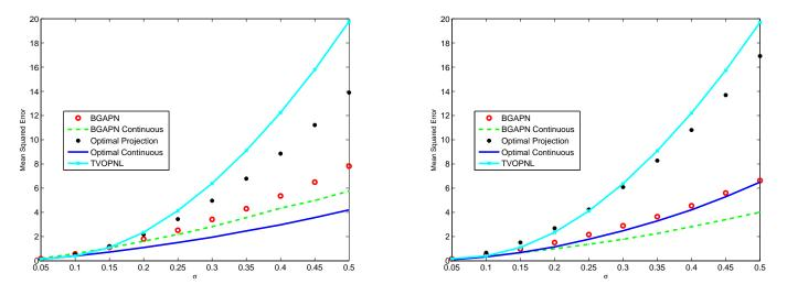
Fig. 3. MSE of the recovered piecewise linear functions (left) and piecewise second-order polynomial functions (right) as a function of the noise variance  $\sigma$  for the methods BGAPN with and without the continuity constraint and the optimal approximation with and without continuity post-processing. As a reference we compare to the non local overparameterized TV (TVOPNL) approach introduced in [38].
