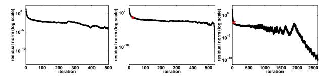
Figure 1: Ltridiag500 residual norm. From left to right k = 0, 1, 20% n. The fault point is marked by the red cross.
