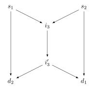
FIG. 2. The butterfly network with coding functions on the edges.
