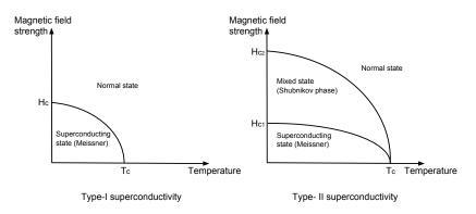
FIG. 2. Sharp transition to the normal state in typ-I superconductors (left plot) and the mixed state in type-II superconductors (right plot).
