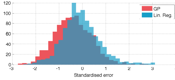
Figure 6. Standardized errors for the GP and linear regression-based emulators for predictions of the wave 8 simulator runs. Most errors lie within the [-2, 2] interval. The GP emulator's errors have a slight negative bias, and the linear regression emulator errors are slightly skewed towards positive values.
