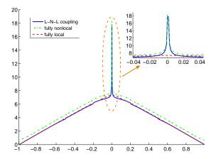
FIGURE 5. The solutions are plotted with mesh size h=1/800, and horizon size  $\delta=0.2$ . We fix the local-nonlocal-local coupling with interfaces at  $x^a=\frac{-1}{2}$  and  $x^b=\frac{1}{2}$ . Kernel function is chosen to be  $\gamma_\delta(x)=\frac{3}{2\delta^3}\chi_{(-\delta,\delta)}(x)$
