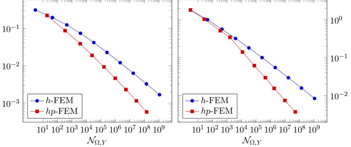
Figure 2:  $\|y^{\frac{s}{2}} \nabla(u - u_h)\|_{L^2(C)}$  for  $s = 0.2$  (left) and  $s = 0.8$  (right) over the total number of degrees of freedom  $\mathcal{N}_{\Omega, Y}$ .
