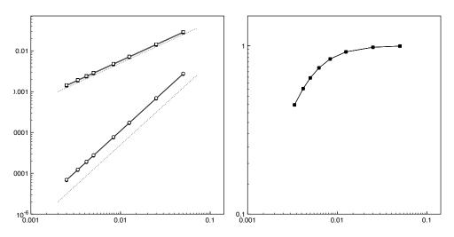
FIG. 5.3. Relative error against mesh size. k = 1, from left to right: n = 1, n = 5. Square markers indicate  $H^1$ -seminorm errors, circle markers indicate  $L^2$ -errors, filled markers indicate global errors and not filled markers indicate local errors. Dotted reference lines (left plot): top y = O(h), bottom  $y = O(h^2)$
