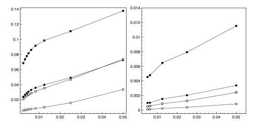
FIG. 5.6. Relative error against mesh size for case 2. From left to right: k = 1 and k = 2. Square markers indicate  $H^1$ -seminorm errors, circle markers indicate  $L^2$ -errors, filled markers indicate global errors and not filled markers indicate local errors.
