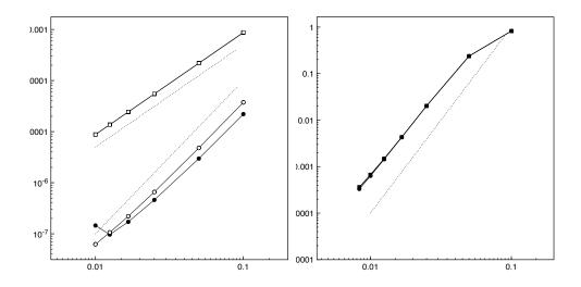
FIG. 5.4. Relative error against mesh size. k = 2, from left to right: n = 1, n = 5. Square markers indicate  $H^1$ -seminorm errors, circle markers indicate  $L^2$ -errors, filled markers indicate global errors and not filled markers indicate local errors. Dotted reference lines (left plot): top  $y = O(h^2)$ , bottom  $y = O(h^3)$ , (right plot)  $y = O(h^2)$
