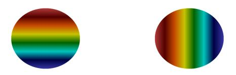
Figure 4: *x*-component (left) and *y*-component (right) of the eigenfunction  $\mathbf{u}_{h,1}$  on the unit disk associated to the eigenvalue  $\kappa_1 = 0$ . The computations are performed on a grid comprising of triangles.
