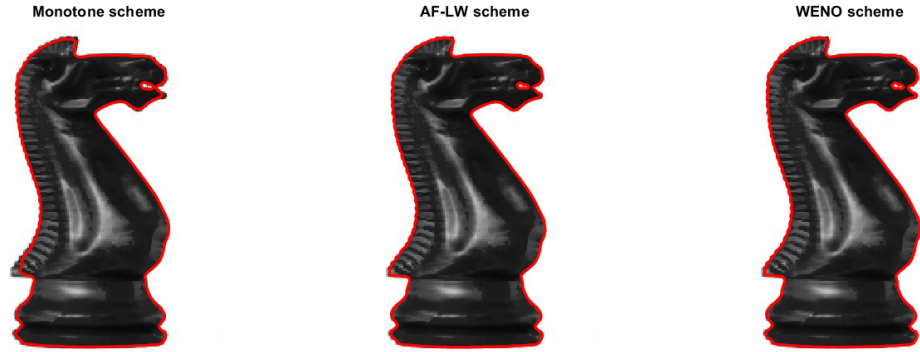
Figure 9: Test 3a with Datum 1. Plots of the final front using the monotone scheme, N_i = 508 (left), the AF-LW scheme, N_i = 544 (middle), and the WENO scheme, N_i = 523 (right), with L^1 norm and tol = 0.000025 , \mu = 2 , K_{reg} = 5 , and velocity \tilde{c} .
