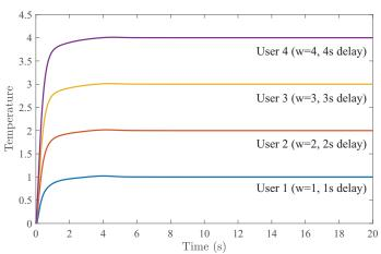
Fig. 3. A Matlab simulation of the step response of the closed-loop temperature dynamics  $(T_{2i}(t))$  for System (8) with 4 users  $(w_i$  and  $\tau_i$  as indicated) coupled with the controller from Theorem 12 with closed-loop gain of .36
