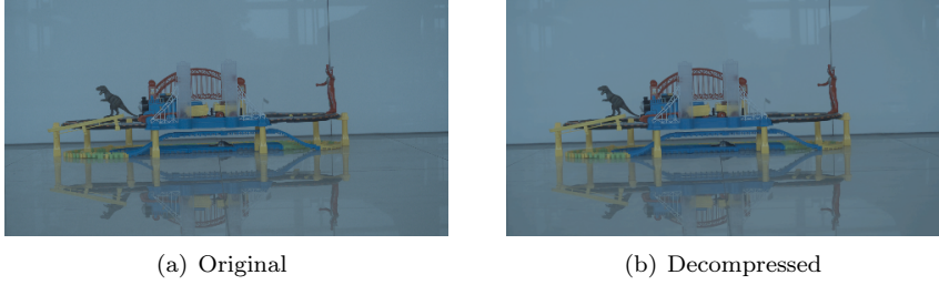
FIG. 2.5. (color online) The RGB frames from the original and the decompressed raw-bayer frames are presented in the left and right panels, respectively. The metrics between these two are: PSNR = 38.94 , SSIM = 0.950 . The dimensions of both images are [2048, 3864, 3] .
