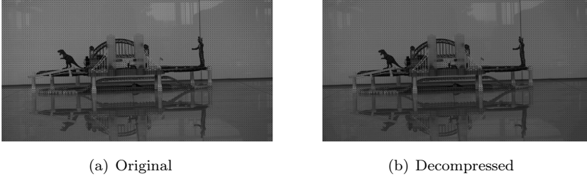
FIG. 2.2. The original and the decompressed raw-bayer images are presented in the left and right panel, respectively. The dimensions of both images are [2048, 3864] . The metrics of the decompressed relative to the original raw-bayer image are: PSNR = 41.64 , SSIM = 0.993 .
