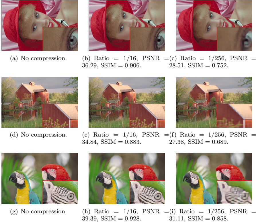
FIG. 2.9. (color online). Comparison of three Kodak RGB images with different compression levels are presented. The left panels present the original Kodak RGB images. The middle panels present the reconstructed RGB images after being compressed by kernel of dimension [8, 8, 1, 4] . The right panels present the reconstructed RGB images after being compressed by kernel [32, 32, 1, 4] . The compression ratios and metric relative to the original RGB images are presented in the panels. Parts of the full images are zoomed in and presented in the red boxes on the bottom right of each panel to demonstrate the reconstruction-quality drop as more compression are carried out.
