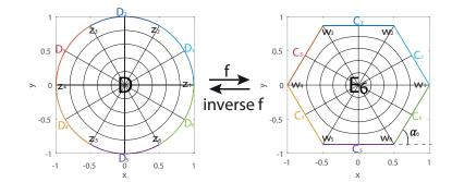
Fig. 2: Schwarz-Christoffel mapping f from a unit disc to a regular hexagon and inverse mapping  $f^{-1}$  from a regular hexagon to a unit disc.
