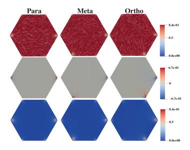
Fig. 10: The images in the first row show the Ortho, Meta and Para solutions of (2.9) with  $\lambda^2 = 2250$ . The images in the second and third rows show  $P_{11}^{2250}P_{12}^{\infty} - P_{12}^{2250}P_{11}^{\infty} = s^{2250}s^{\infty}\sin((2\gamma^{\infty} - 2\gamma^{2250}))$  and  $(\mathbf{P}^{\infty})^2/2 - (\mathbf{P}^{2250})^2/2 = (s^{\infty})^2 - (s^{2250})^2$ , respectively.
