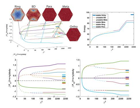
Fig. 11: Bifurcation diagram for reduced LdG model in regular hexagon domain. Top left: plot of  $\int P_{11} (1 + x + y) dx dy$ ,  $\int P_{12} (1 + x + y)$  verses  $\lambda^2$ ; top right: plot of the energy in (3.24) verses  $\lambda^2$ ; bottom: orthogonal 2D projections of the full 3D plot.
