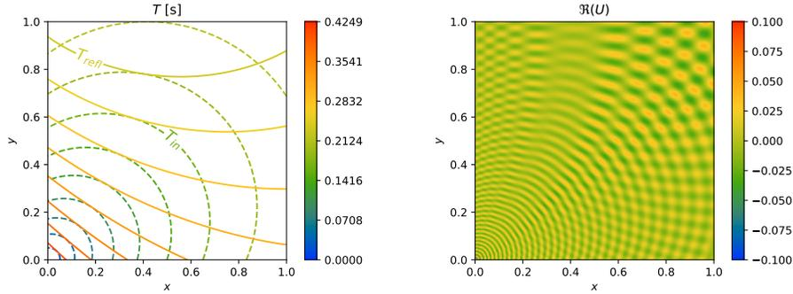
FIG. 8.2. A single reflection from a wall in a semi-infinite domain for  $\omega = 1000$  (we consider only the top edge of the boundary to be reflecting). Left:  $T$  for the incident and reflected fields. The reflected field satisfies a specular reflection condition along the edge of the domain. Right: the real part of the approximation to the solution of the Helmholtz equation so obtained, given by (8.15).
