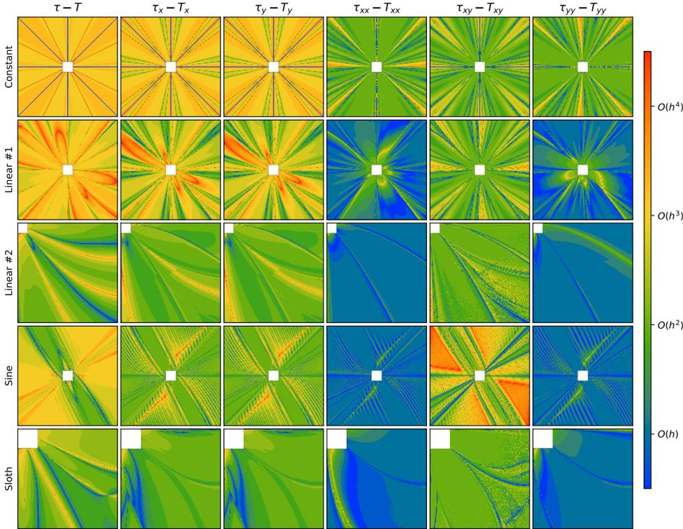
FIG. 8.6. A plot of the pointwise convergence at each point in  $\Omega_h$  for *JMM4*. To obtain these plots, starting with  $N = 129$ , we decimate each larger problem size (up to  $N = 2,049$ ) to a  $129 \times 129$  grid, and do a least squares fit at each point. This gives us an estimate of the order of convergence at each point.
