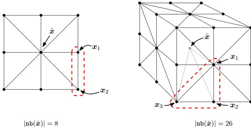
FIG. 5.1. The neighborhoods typically used by semi-Lagrangian solvers in 2D and 3D on a regular grid. These are the stencils used by Tsitsiklis’s algorithm and two of the OLIM stencils [46, 30]. Left: “olim8” in  $\mathbb{R}^2$ . This is the 8-point stencil used in this paper. Right: “olim26” in  $\mathbb{R}^3$ .
