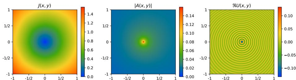
FIG. 8.7. Plots related to computing the amplitude and a numerical approximation to the solution to  $(\Delta + \omega^2 s(\mathbf{x})^2)u(\mathbf{x}) = \delta(\mathbf{x})$ , denoted  $U(\mathbf{x})$  for the Linear #1 test problem. Left: the geometric spreading. Middle: the amplitude function. Right: the numerical solution  $U$ .
