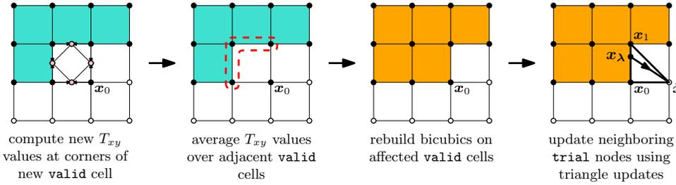
FIG. 7.2. Local cell marching. After computing values of  $T_{xy}$  as shown in Figure 7.1 (left), to ensure continuity of the global interpolant, nodal values incident on the newly valid cell (containing  $\mathbf{x}_0$ ) can be recomputed by averaging over  $T_{xy}$  values taken from incident valid cells (middle). Finally, a bicubic cell-based interpolant is constructed (right).
