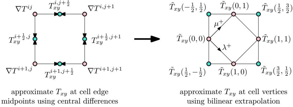
FIG. 7.1. Cell-based interpolation. To approximate the mixed second partials of a function with  $O(h^2)$  accuracy from  $O(h^3)$  accurate gradient values available at the corners of a cell, the following method of using central differences to approximate the mixed partials at the midpoints of the edges of the cell, followed by bilinear extrapolation, can be used.
