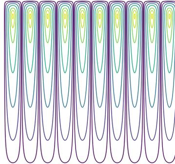
FIGURE 2. Skewed tall and thin convection rolls.
