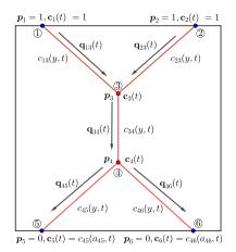
Fig. 10: 2D schematic of a reflected-Y network with labelled physical quantities presented in §3.
