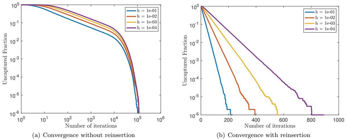
FIG. 8. *Convergence statistics of the KMC method for the simplified problem (4.36). Left: In the absence of reinsertion, a polynomial rate of convergence is attained shown by the linear behavior on the log-log plot. Right: Reinsertion recovers exponential convergence as seen in the linear behavior on the log plot. Simulations based on ensemble of  $10^6$  particles.*
