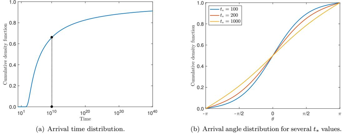
FIG. 5. CDFs of arrival time and location for the reinsertion step when  $D = 1$ ,  $\mu = 60$ . Left: The reinsertion time distribution  $F_\theta(\tau) = \int_0^\tau \chi_0(\eta) d\eta$  given by (1.2) (dashed line indicates the cutoff  $\tau = 10^{10}$  after which the fitted density (4.33) is used). Right: The arrival location CDF (4.34) for several arrival times  $\tau_*$ . The distribution is largely uniform for large  $\tau_*$ .
