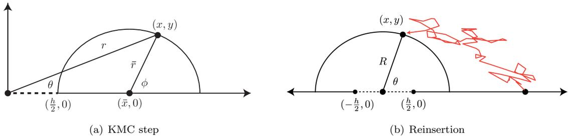
FIG. 6. A schematic showing the simplified KMC solution in the upper half plane. (a) the projection step from the real line back into the bulk. (b) The reinsertion step to keep the particle in the vicinity of the absorbing set.
