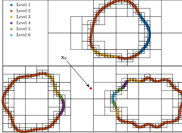
FIG. 3. Visualization of the tree based particle-in-cell method for efficient evaluation of the distance  $d(\mathbf{x}_0, \partial\Omega)$ . The coloring of each point indicates the highest grid level that the vertex of  $\partial\Omega$  is considered for the closest point evaluation. If the maximum refinement level is  $k$ , then all points in levels  $1, 2, \dots, k-1$  are excluded from the distance calculation of  $d(\mathbf{x}_0, \partial\Omega)$ .
