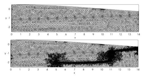
FIG. 4.11. Example III: Initial and final adaptively refined meshes.
