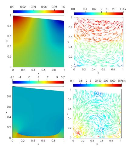
FIG. 4.4. Example II: Primal (top) and adjoint (bottom) pressure and velocity approximations on the final mesh.
