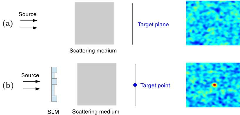
FIG. 1.1. *Focusing wave through a scattering medium. Without any control one gets a speckle pattern in the target plane (a). With a spatial light modulator (SLM) one can focus on a target point by imposing appropriate phase shifts (b) [From [16]].*
