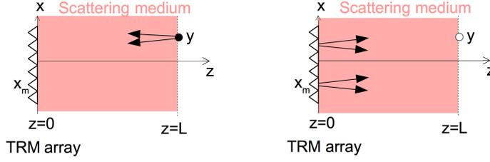
FIG. 3.1. *Time-reversal experiment. Left: first step of the experiment (a point source transmits from  $(\mathbf{y}, L)$  and the TRM in the plane  $z = 0$  is used as an array of receivers). Right: second step of the experiment (the TRM is used as an array of sources).*
