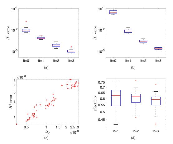
Figure 9: nonlinear problem; adaptive enrichment. (a)-(b) boxplots of the relative  $H^1$  error on the test set for smooth and Gaussian sampling of localized BCs. (b) correlation between  $\Delta_{\mu}$  and relative  $H^1$  error (smooth sampling). (c) out-of-sample effectivity of the error indicator  $\Delta_{\mu}/E_{\rm rel}$  (27) (smooth sampling).
