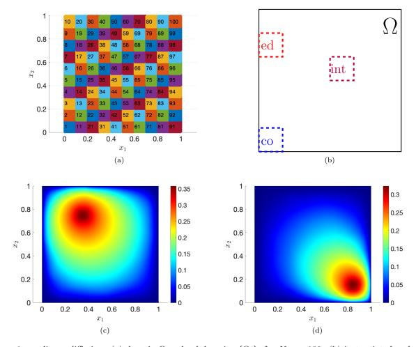
Figure 1: nonlinear diffusion. (a) domain  $\Omega$  and subdomains  $\{\Omega_i\}_i$  for  $N_{\rm dd}=100$ . (b) instantiated archetype components. (c)-(d) solution fields for  $N_{\rm dd}=100$  and two choices of the parameters.
