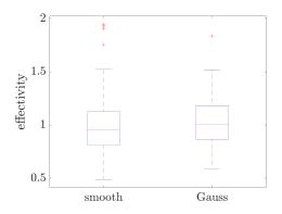
Figure 5: linear problem. Effectivity of the error indicator  $\eta = \frac{\widehat{E}(n_{\text{test}}=10)}{\widehat{E}(n_{\text{test}}=100)}$  for 100 independent runs and for both Gaussian and smooth training.
