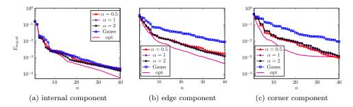
Figure 7: nonlinear problem. Local approximation errors (45) for three choices of  $\alpha$  ( $N_{\rm f} = 20$ ,  $\bar{u}_{\rm max} = 0.5$ ), and for Gaussian sampling (44).
