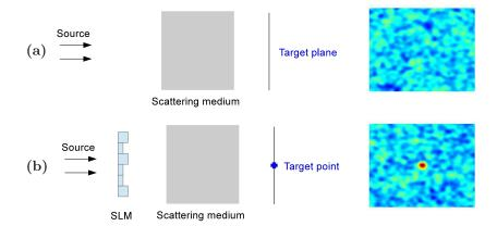
Fig. 1.1. Focusing wave through a scattering medium. Without any control one gets a speckle pattern in the target plane (a). With a spatial light modulator (SLM) one can focus on a target point by imposing appropriate phase shifts (b) [From [16]].
