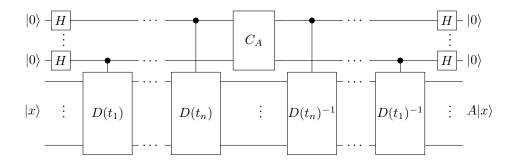
Figure 3: Quantum circuit implementing a linear combination
