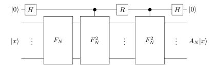
Figure 1: Circuit realizing a quantum Hartley transform
