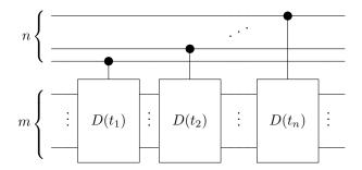
Figure 2: Quantum circuit for a transversal case operator
