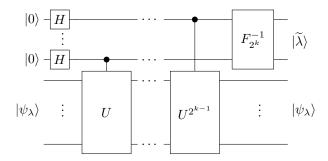
Figure 4: Quantum circuit for eigenvalue estimation
