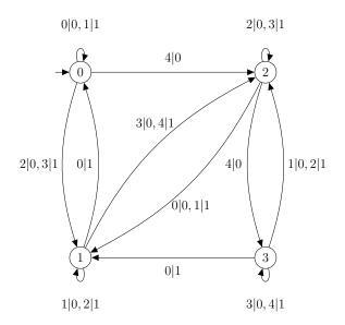
Figure 1: The transducer N in base 2 converting  $D_2$  into  $\{0, 1\}$ .
