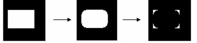
Fig. 4. The morphological residual model. Applying opening on the original image with circle structuring elements, then subtraction of result image from original image can obtain the morphological residuals.
