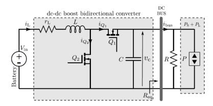
Figure 3. DC MG simplified model in stand-alone operation.
