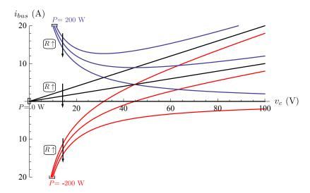
$(v_c, i_{bus})$  characteristics for several values of the parameters P and R. Figure 4.
