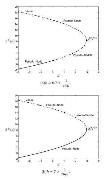
Figure 14. Bifurcation diagrams showing a SN bifurcation with parameters b = 0.06, w = 0.6,  $y_r = 2$  and a = 0.3.
