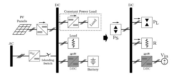
Figure 2. DC MG and its equivalent model in stand-alone operation.
