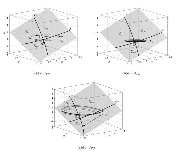
Figure 13. State-space diagrams of system (8) considering w=0.6, b=0.06,  $y_r=2$ , a=0.5 and k=0.5. (a) d=-1.1. (b)  $d=d_{TS}=-1.06$ . (c) d=-1.
