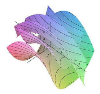
Figure 3: Hyperbolic paraboloid and one of its offsets
