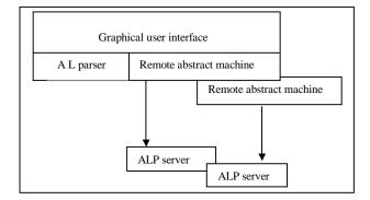
Fig. 11. The structure of Java application
