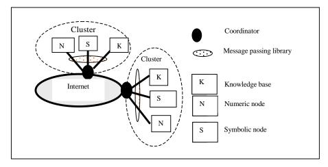
Fig. 1. Architecture of a distributed knowledge base on the Internet
