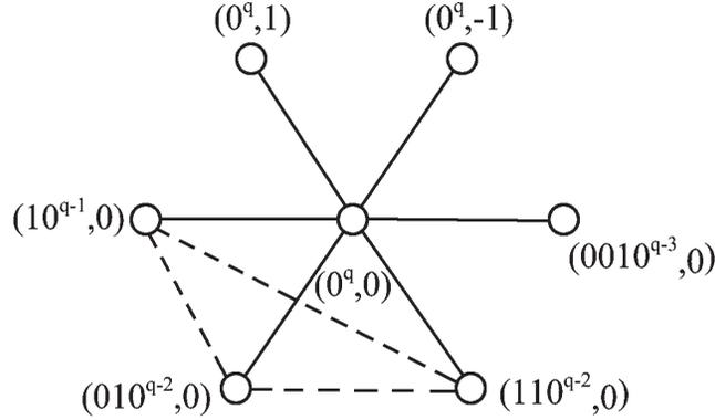
Fig. 2. Connections between node  $(0^q, 0)$  and its neighbors.
