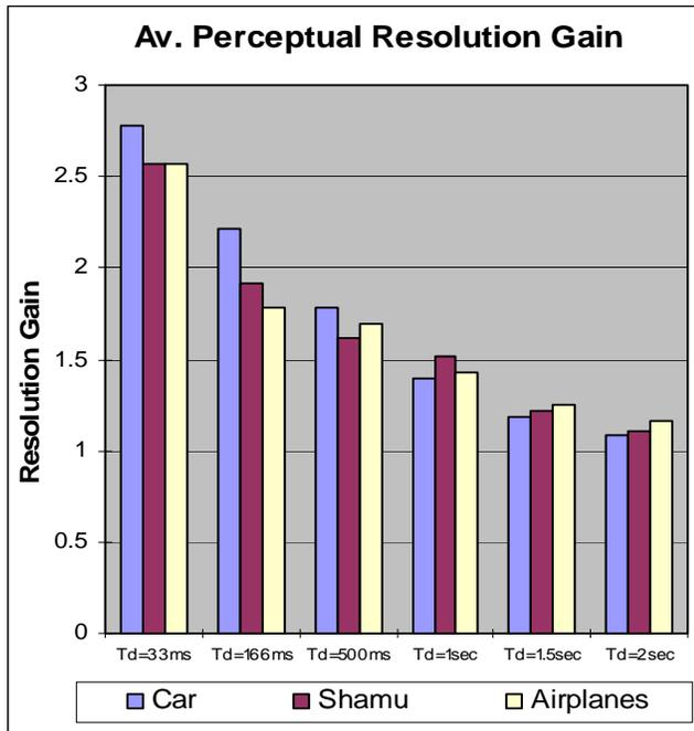
**Figure 12.** Average perceptual resolution gain results for three test videos.
