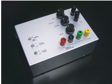
Figure 3: The picture of the exterior of self-made SCR amplifier
