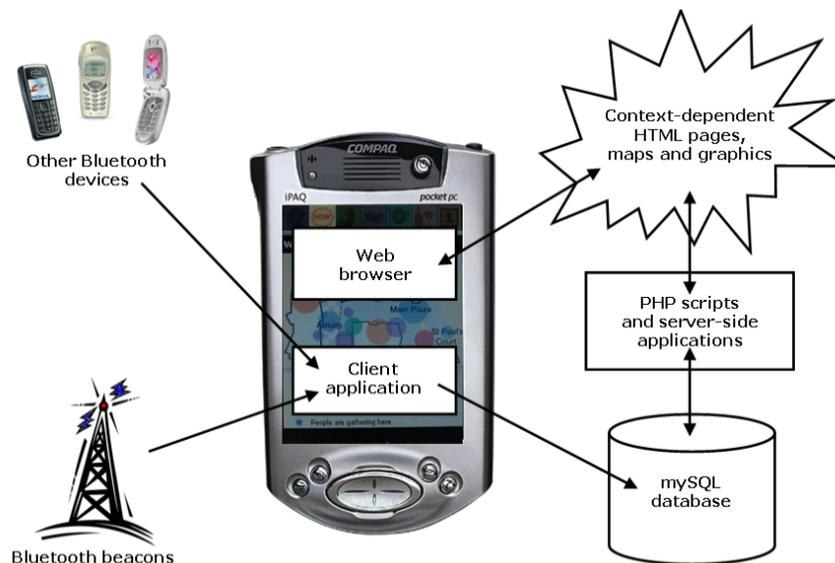
**Figure 3. Just-for-Us prototype system architecture**
