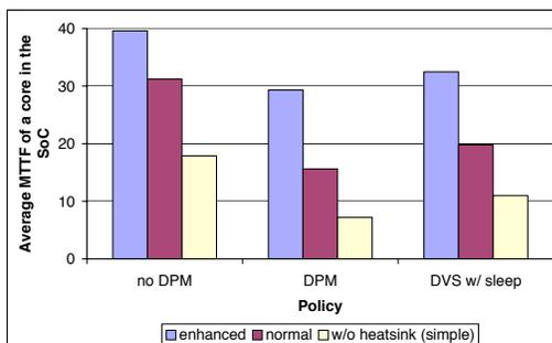
Figure 5: Comparing average MTTF for different thermal packages.
