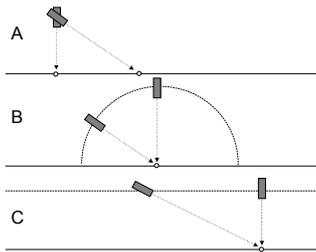
Fig. 2. Three kinds of camera rotation: the panoramic rotation (A), the lunar rotation (B), and the trans-rotation (C).
