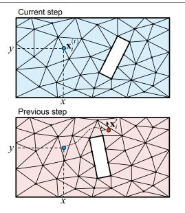
Figure 2: A two-dimensional representation of the generalized semi-Lagrangian advection step. We trace back from the position where a velocity is stored in the new mesh,  $\mathbf{x}_i = (x, y)$ , interpolate the velocity using the old mesh and velocity field, and update the velocity in the new mesh.
