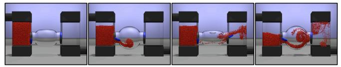
Figure 5: Red particles are transfered from the left tank to the right by squeezing and releasing the central bulb. The blue valves are coupled to the fluid simulation and prevent backflow.
